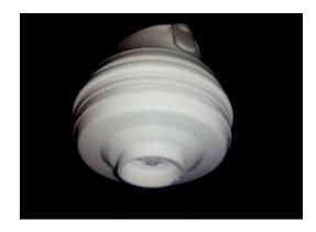
The first picture shows the piston out of the bottle. Note how the top edges flare out slightly to fit securely inside the diameter of the bottle. The product/cream sits on top of the piston as it is shown here inside the bottle cylinder. As the piston rises from the bottom of the bottle, it lifts the product up to the bottom of the engine. Note the design of the middle section of the piston.
